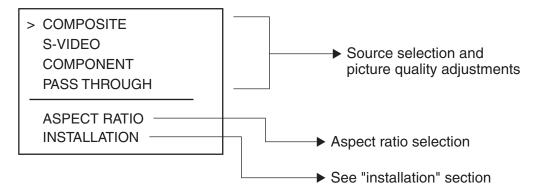
When the MENU button is pressed on either the remote control or the front panel, the main menu will appear on-screen. An example of the main menu is shown above.
